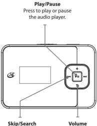
Skip/Search Press to skip. Press and hold to search through tracks. Volume Press to adjust the volume.
